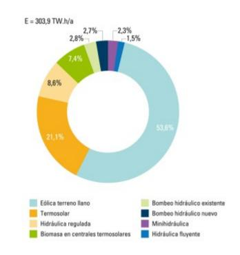
Configuration and electricity generation, mix optimized for NSEC = 500c€/kWh, SM=2.29, SF=99.993%, LEC= 2.42 c€/kWh
