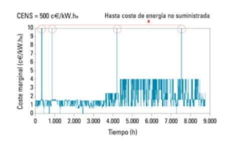
Annual hourly evolution of marginal cost of non-supplied paragral hourly evolution of marginal cost of non-supplied electric for an optimized mix for NSEC = 500 c/kWh, SM= 2.29, SF= 99.993%; LEC= 2.42 c€/kWh
